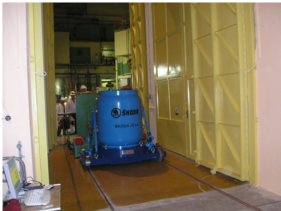
Fig. 12. VPVR/M cask being moved into the storage area
