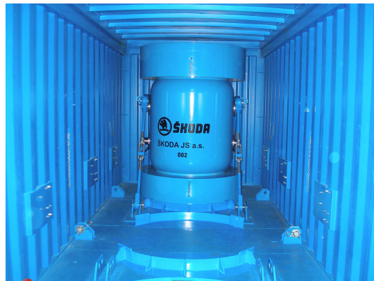
Fig. 13 Interior of the ISO container with one VPVR/M cask
